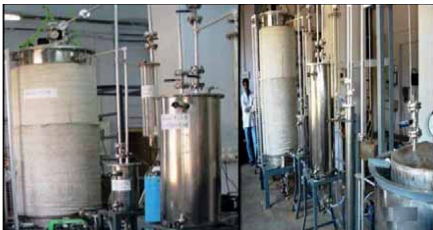
Figure 5: An 800 litre bioreactor plant for biohydrogen production, IIT Kharagpur
